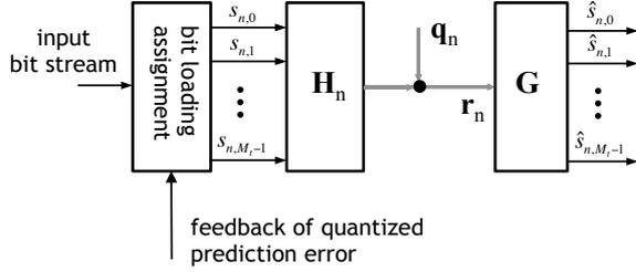
Figure 1: A MIMO system with bit loading feedback.
