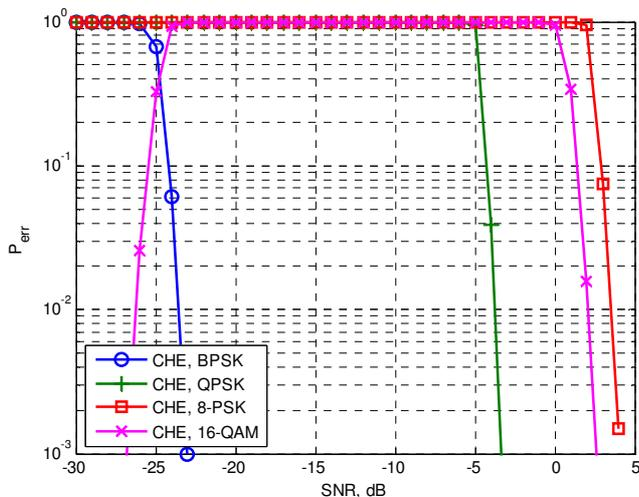
Figure 3. Error probability of recognition (phase averaging with frequency maximization)
