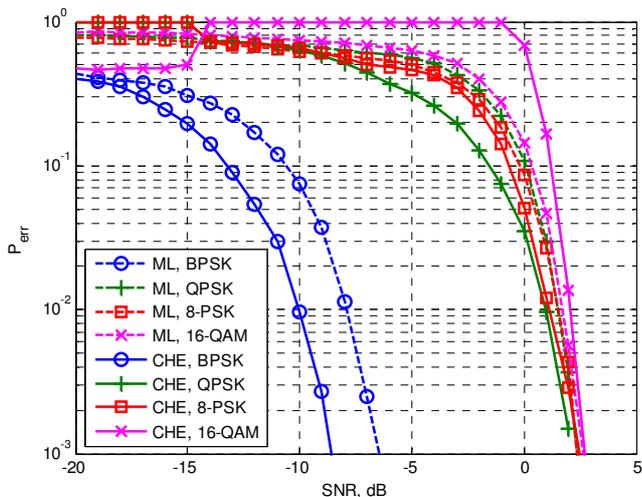
Figure 1. Error probability of recognition (coherent case)
