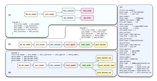
**Fig. 2**: Example Barista networks. (a) The topography of a feature extraction network and the corresponding network specification file. (b) The topography of a decoding network and the corresponding network specification file. (c) The configuration file shared between networks (a) and (b). (d) The network used in the second case study (see section 3.2).
