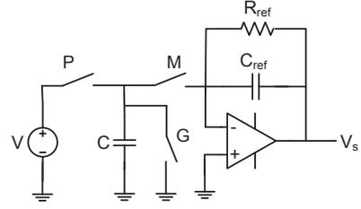
Figure 3. A practical circuit for a charge transfer sensor
