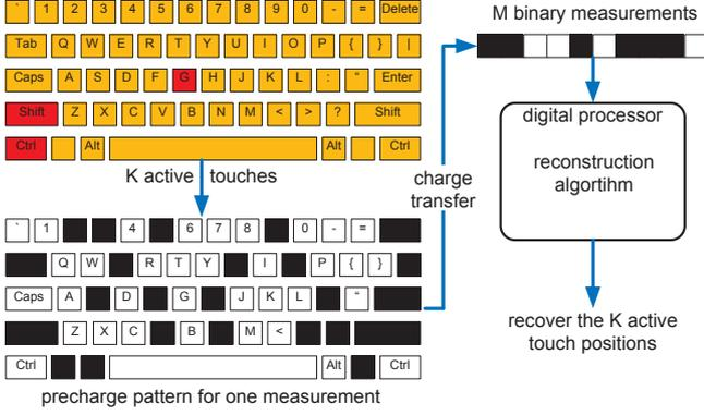
Figure 5. The self-capacitance measurement process with the proposed AFE architecture.
