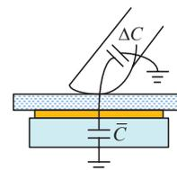
Figure 1. The capacitance change in the presence of a finger.
