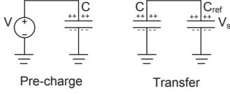
Figure 2. Basic principle of a charge transfer capacitance sensor
