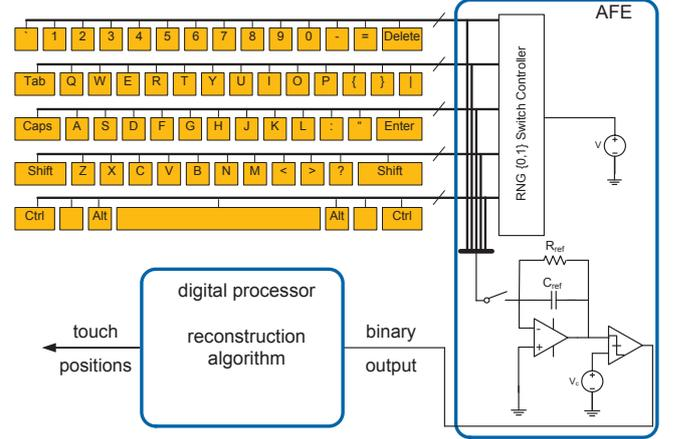
Figure 4. Block diagram of the proposed self-capacitance sensing AFE architecture
