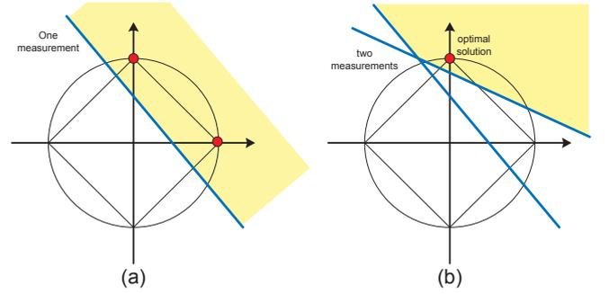
Figure 6. A geometrical interpretation of the 1-bit compressive sensing scheme. (a) one measurement (b) two measurements
