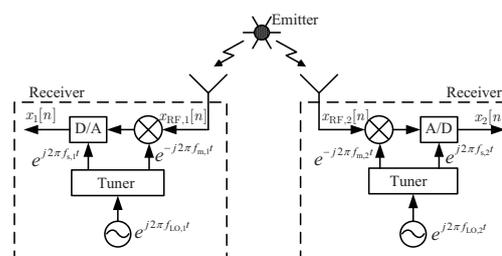
Fig. 1. Incoherent reception in a typical passive system
