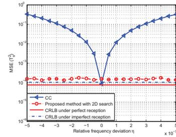
**Fig. 3.** MSE of  $\hat{D}$  with different relative frequency derivation of local clock (SNR=10dB,  $D = 3.2T_s$ )
