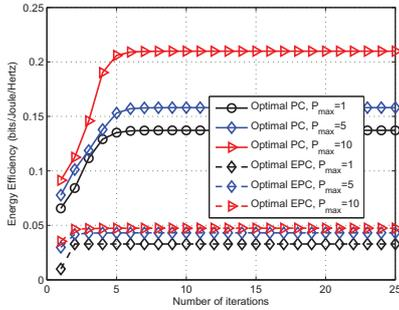
Fig. 2. Convergence of the proposed power allocation algorithm.
