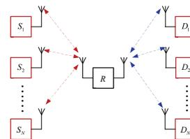
Fig. 1. A multiuser two-way relay network.
