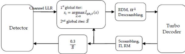
Figure 6 Online GMI based forward scaling and uniform backward scaling for IDD.
