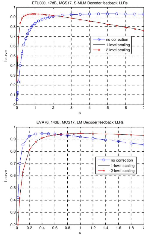
Figure 5 I-curves of decoder extrinsic output LLR without applying online GMI scaling to detector output
