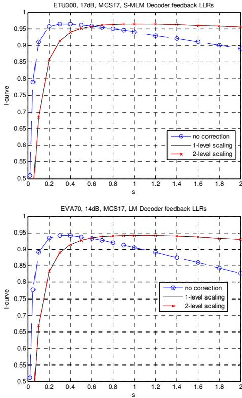
Figure 4 I-curves of decoder extrinsic output LLR after applying online GMI scaling to detector output
