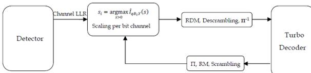
Figure 2 Decoder decision based scaling for detector output LLRs for 1<sup>st</sup> global iteration.
