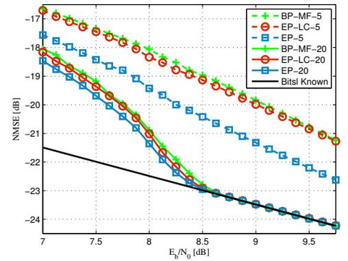
**Fig. 3.** Channel taps NMSE versus  $E_b/N_0$ ; dashed curves refer to 5 turbo iterations; solid curves refer to 20 turbo iterations.
