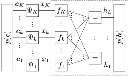
**Fig. 1.** Factor graph of an OFDM system with  $K$  subcarrier and  $L$  channel taps.
