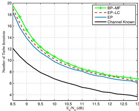
**Fig. 4.** Average number of turbo iterations versus  $E_b/N_0$ .
