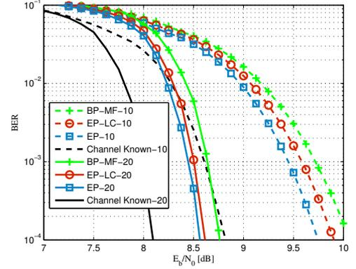
**Fig. 2.** BER versus  $E_b/N_0$ ; dashed curves refer to 10 turbo iterations; solid curves refer to 20 turbo iterations.
