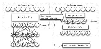
Fig. 1. Diagram of the low-rank factorized DNN.
