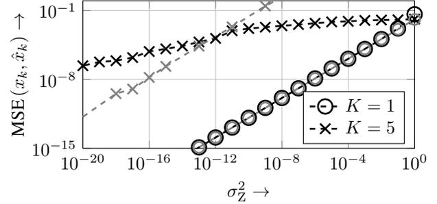
**Fig. 2.** Comparison of simulation results (via ESPRIT, black) and CRB (grey) for  $K$  pulses,  $|\mathbb{L}| = 2K + 1$ , unit power filter kernel,  $M = |\mathbb{L}|$ .
