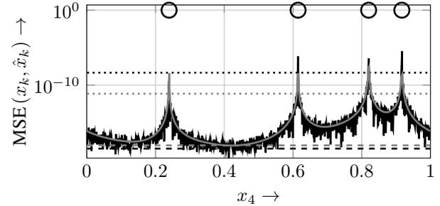
**Fig. 3.** Comparison of simulation results (via ESPRIT, black) and CRB (grey);  $K - 1 = 4$  pulses on fixed positions (circles);  $x_4$  changes on x-axis; solid lines: MSE dependent on  $x_4$ ; dotted lines: average of MSE for all positions  $x_4$ ; dashed lines: MSE by omitting  $x_4$ ;  $M = |\mathbb{L}| = 11$ ;  $\sigma_z^2 = 10^{-15}$
