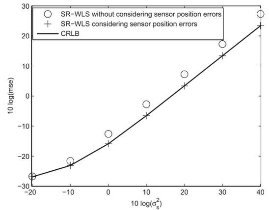
**Fig. 3.** Range (TOA) localization performance of SR-WLS considering sensor position errors, under the 200 random geometries.
