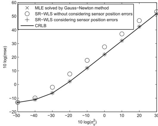
**Fig. 2.** Range (TOA) localization performance of SR-WLS considering sensor position errors, under the specific geometry in Table 1.
