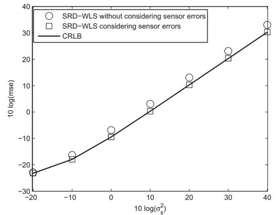
**Fig. 5.** Range difference (TDOA) localization performance of SRD-WLS considering sensor position errors, under the 200 random geometries.
