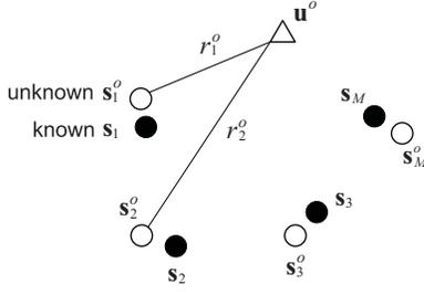
**Fig. 1.** Localization scenario. Open circles are the true sensor positions and closed circles are the available sensor positions.
