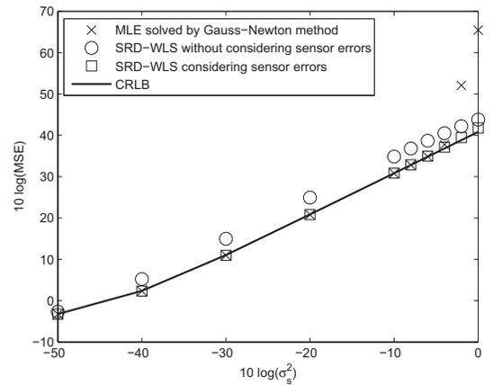
**Fig. 4.** Range difference (TDOA) localization performance of SRD-WLS considering sensor position errors, under the specific geometry in Table 1.
