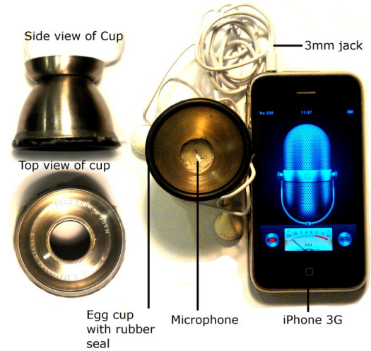
Figure 1: Hand-made stethoscope, made with an aluminium egg-cup and the microphone from a mobile phone hands-free kit plugged into an iPhone 3G.
