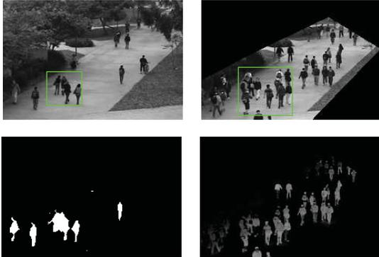
**Fig. 2.** Examples of scene. Left top image shows the 100th frame with largest crowd bounding box while segmentation of crowd area is shown in left bottom image. Right top image shows a frame with ROI mask, and the normalized complement image is shown in the right bottom.
