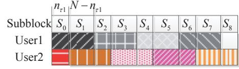
Fig. 2. Subblock segmentation for a 2-user  $2 \times 1$  MISO channel
