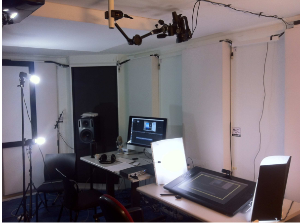
Fig. 1. The recording studio for the DSP class—a modern version of the classroom. The instructor teaches on the tablet, while an overhead camera records the instructor's hand. Then, the video and audio streams are merged and edited in the workstation.
