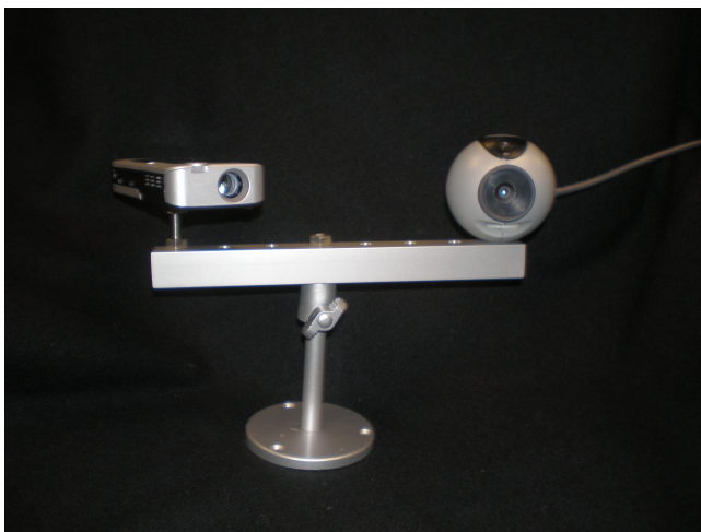
Fig. 4. Our experimental set up is composed of a micro-LED projector and an offset visible light camera.
