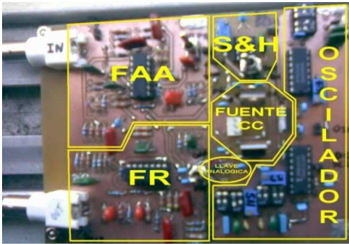
Figure 2. Sampling and reconstruction circuit board of Fig.1 Block Diagram
