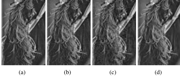
Fig. 2. Experimental results: (a) original image, (b) simulated degraded image with AWGN (15dB), (c) reconstructed image using the OMP method, and (d) reconstructed image using the proposed method.
