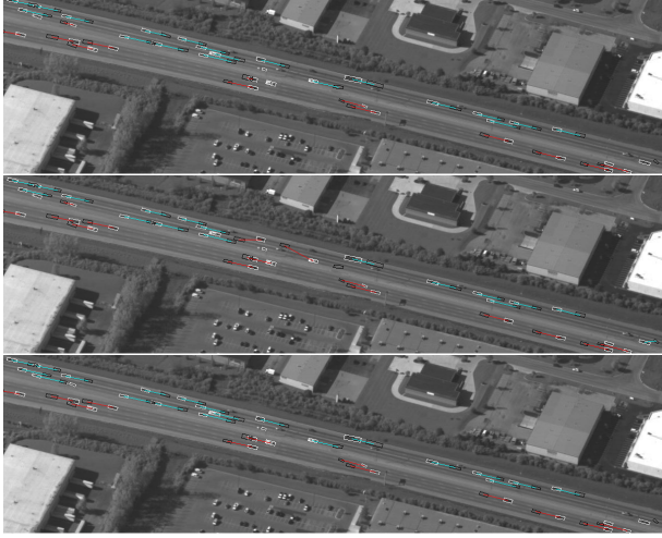
Fig. 3. Associations with different contexts on Sequence 1. Top: NoCon. Middle: SC. Bottom: MCC. Black(White) rectangle: detection in the last(current) frame. Red(blue) line: rightward(leftward) association output.
