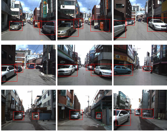
Fig. 5. Results for vehicle detection by using the proposed method with a Gaussian process classifier
