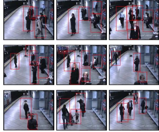
Fig. 7. Results for pedestrian detection by using the proposed method with a support vector machine
