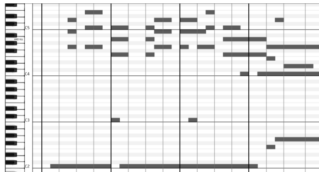
Fig. 3. Example of transcription based on pulses using q = 2 (quantization to a eighth note) in a 4/4 meter.
