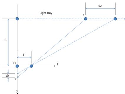
**Fig. 3.** Geometric relationships in a structured light setup.
