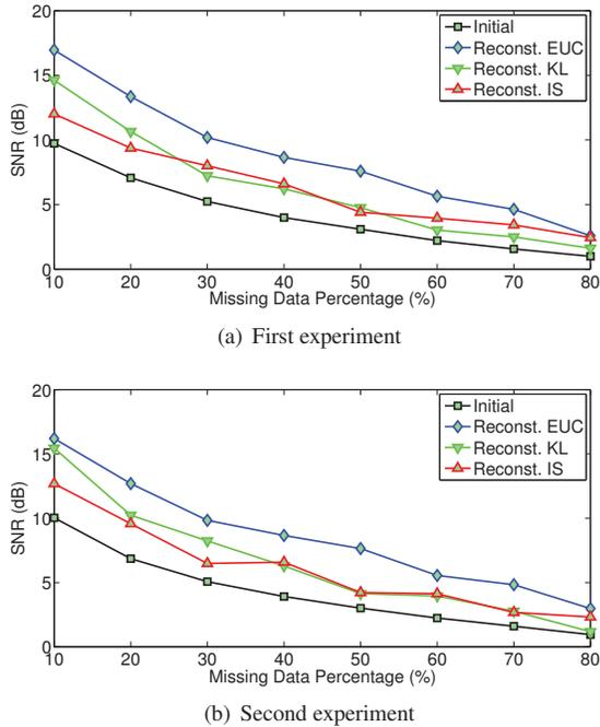
**Fig. 2.** Results of the experiments. As side information ( $X_2$ ), we used a) own transcriptions of the test files, b) *different* transcriptions of other test files. Initial SNR is computed by substituting 0 as missing values.
