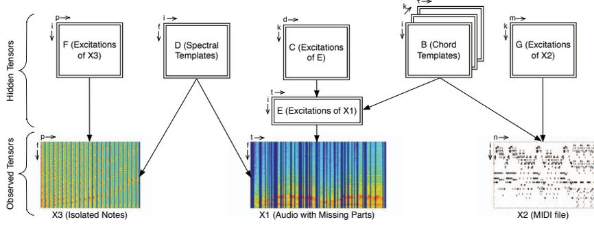
**Fig. 1.** General sketch of the proposed approach. The idea is to incorporate information from the recordings of the instrument and a score of the same genre. The blocks visualise the tensors that are defined in the model and the relation between them. The lower-case letters and arrows near the blocks represent the indices of a particular tensor.
