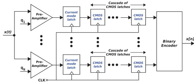
Fig. 2. Schematic of a bit-error optimised flash ADC.
