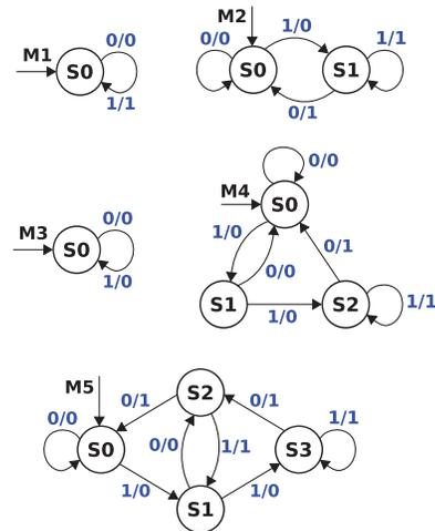
Fig. 4. FSM abstractions automatically generated by DAE2FSM for the CML, and for cascades of two and three latches, operating under  $V_{DD} = 0.8V, 1.0V$ , and  $1.2V$ . For more details, please see Fig. 5.
