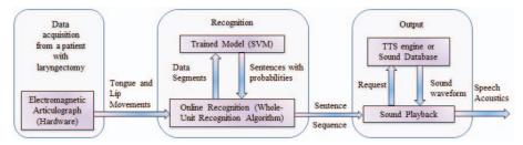
Fig. 1. Design of the EMA-based silent speech interface
