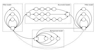
Fig. 1. General scheme of acoustic KWS.
