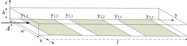
**Fig. 1:** An equally spaced linear array of three biosensors in a rectangular flow chamber. The fluid containing target molecules enters from the left side. The concentration of target molecules at the inlet is  $A^*$  as expressed in the boundary condition (4).
