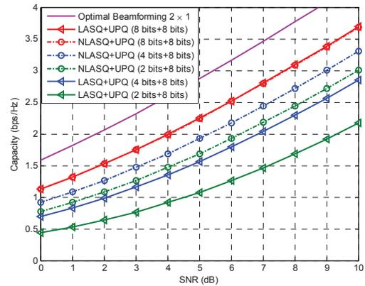
Fig. 3. Capacity of scenario 2 & 3 for MISO beamforming systems.
