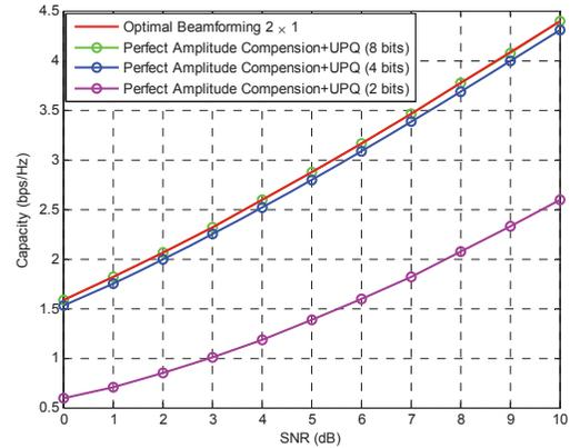
Fig. 2. Capacity of scenario 1 for MISO beamforming systems.
