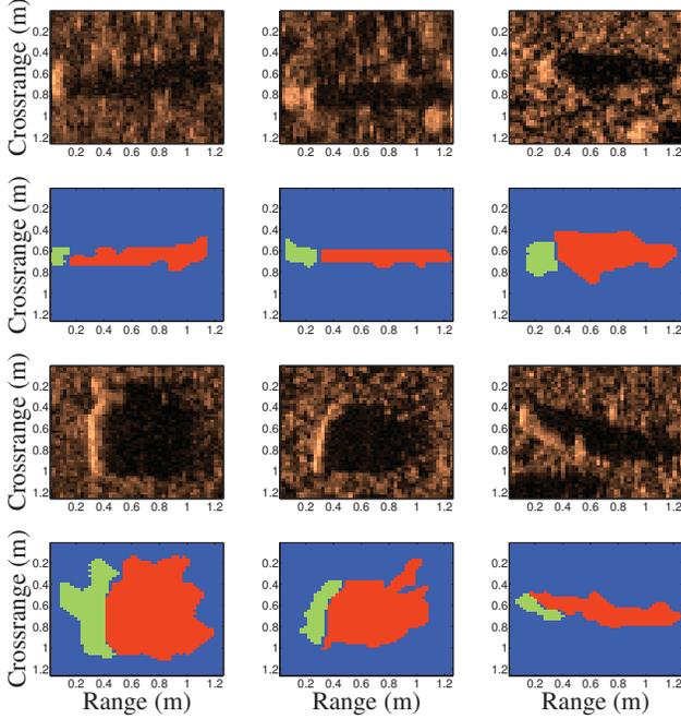
**Fig. 1.** The first row shows three snapshots of spherical mines. The second row illustrates their segmentation into three regions: highlight (green), shadow (red) and background (blue). the third row depicts three cylindrical mines and the forth row the corresponding segmentation results.
