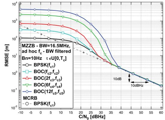
Fig. 2: Multi-peaks effect - filtered BOC modulations.
