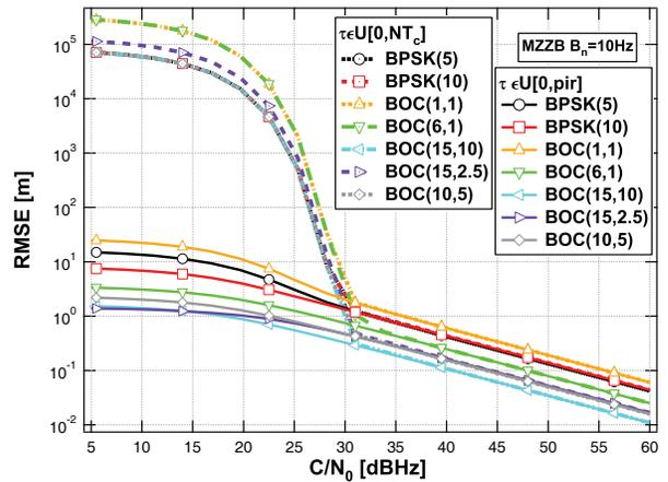
Fig. 3: Theoretical acquisition and tracking performance of Galileo GNSS by means of MZZB.
