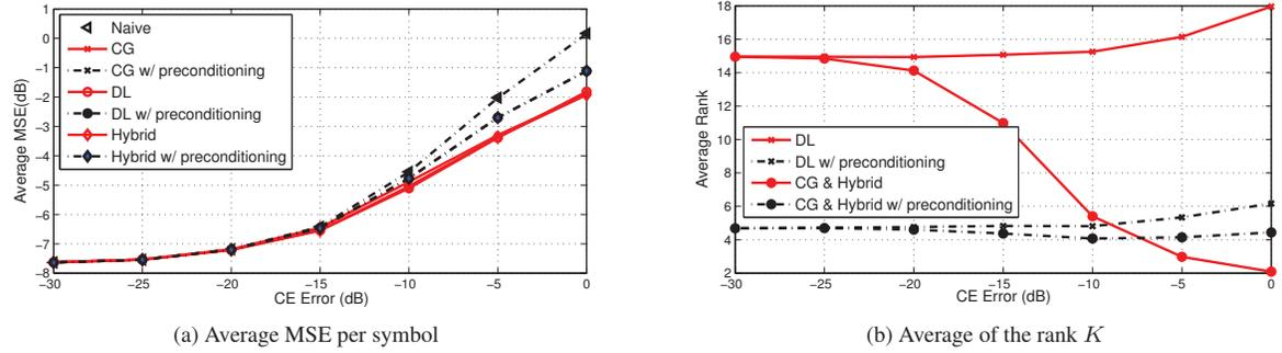
**Fig. 2:** Serial equalization for multipath channels with the same parameters as those in Fig. 1 except  $\hat{\sigma}_n^2 = \sigma_n^2$ . Preconditioning reduces the complexity with minor performance degradation when the CE is accurate. Without preconditioning, the CG, DL and hybrid schemes achieve similar performance, with DL performing slightly better.
