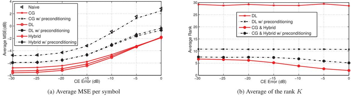
**Fig. 1:** Serial equalization for multipath channels with  $n_t = n_r = 2$ ,  $L = 20$ ,  $Q = 6$ ,  $T = 128$ ,  $M = 294$ ,  $N = 256$ ,  $\text{SNR} \triangleq 1/\sigma_n^2 = 10$  dB,  $\hat{\sigma}_n^2 = 0$  and decision delay  $T_d = 64$ . The DL scheme outperforms CG but requires higher complexity. Preconditioning degrades performance.
