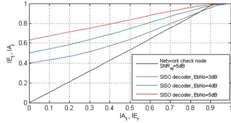
**Fig. 2.** EXIT chart of JNCD algorithm over Fully-Interleaved fading channels
