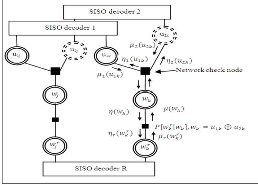
**Fig. 1.** Factor graph of JNCD algorithm.
