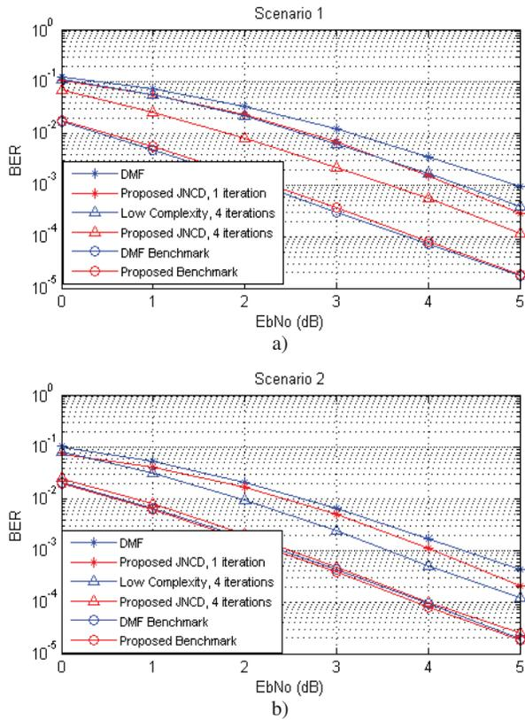
**Fig. 3.** Performance of the proposed JNCD algorithm compared with DMF algorithm in [9]
