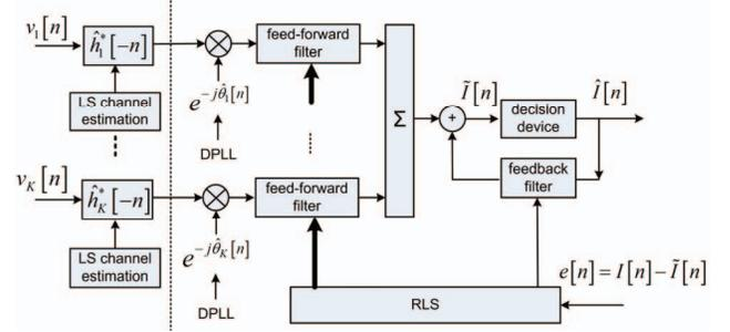
Fig. 2. The receiver structure of PPC-McDFE.
