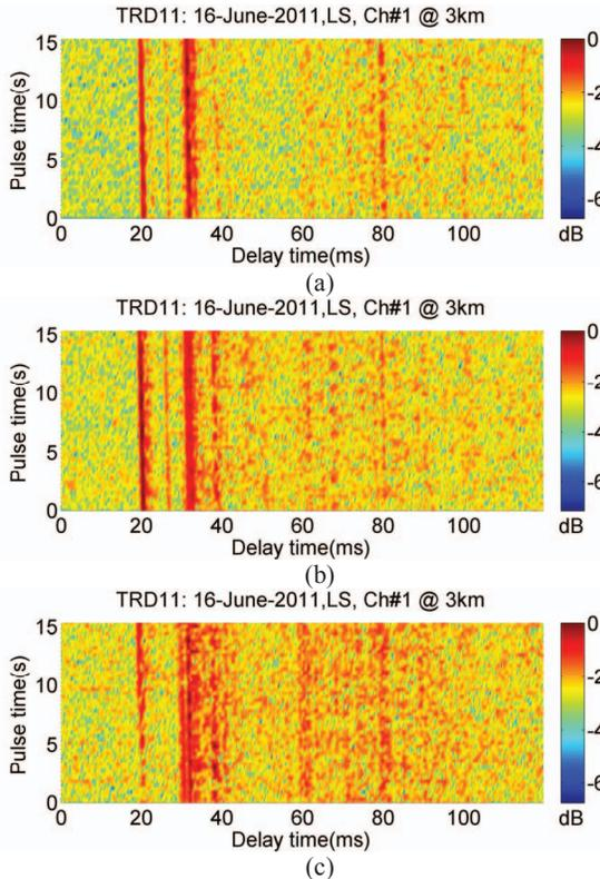
Fig. 6. Channel impulse response estimated by the LS method. (a) The 1st period. (b) The 9th period. (c) The 15th period.
