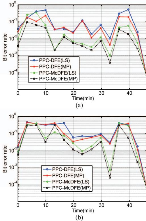
**Fig. 8.** The receiver performance in terms of BER. (a) 1 kbps. (b) 2 kbps.
