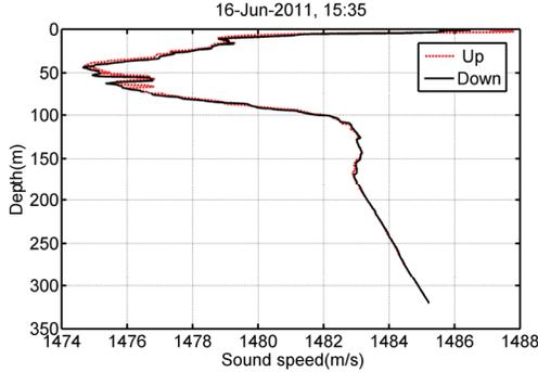
Fig. 5. Sound speed profile measured by the R/V Gunnerus.
