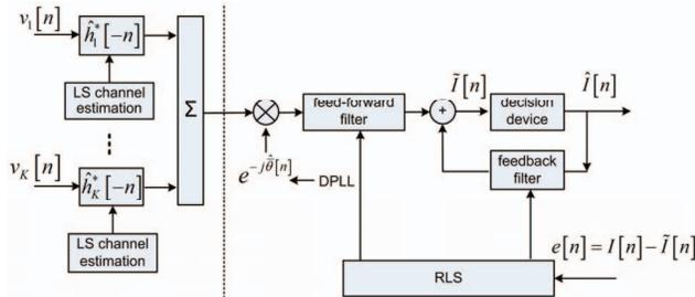
Fig. 1. The time reversal receiver structure PPC-DFE.
