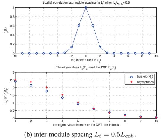
**Fig. 2.** Effectiveness of the asymptotic results in approximating the eigen-results in a 20-module array system. Parameters in use: number of modular arrays  $L = 20$ , in (a) inter-module spacing  $L_t = 0.25L_{coh}$ , in (b) inter-module spacing  $L_t = 0.5L_{coh}$ .
