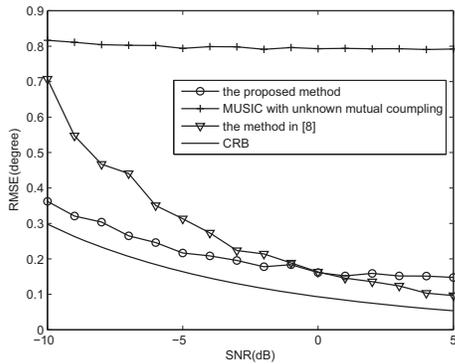
Fig. 2 RMSE of the DOA estimates versus SNR. The number of snapshots is 500.
