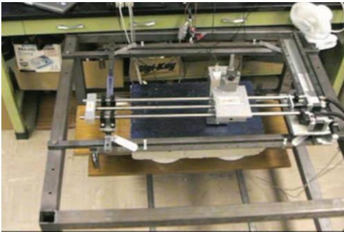
**Fig. 2.** Near-field monostatic stripmap SAR imaging system at Missouri S&T.
