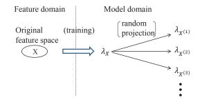
**Fig. 3**. Random projection on the acoustic model domain. An acoustic model is transformed using various random matrices.
