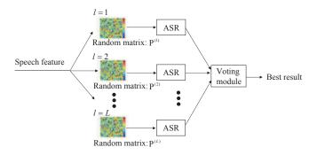
Fig. 4. Vote-based combination for decoding
