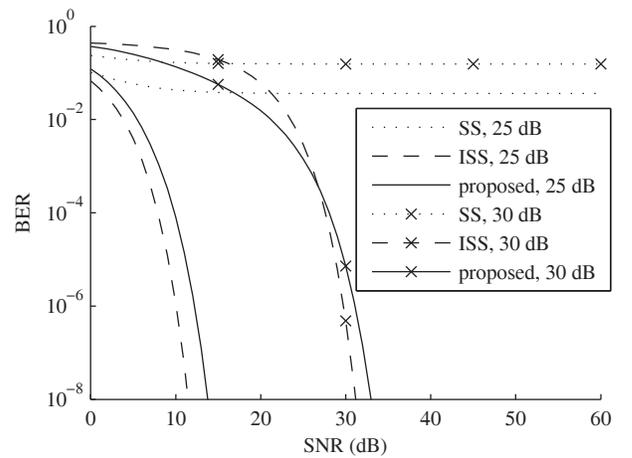
**Fig. 3.** BER vs. SNR under different SWRs (25 and 30 dB), for SS, ISS ( $\lambda = 1$ ), and the proposed scheme.  $N = 1024$ .
