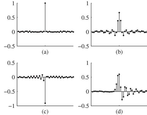
**Fig. 1.** Normalized correlation between the processed PN sequence and the reference ( $N = 8192$ ). (a) no processing; (b) MP3 compression at 96 kbps; (c) playing and recording via sound card; (d) lowpass filtering with a cutoff frequency of 12 kHz. Only a few samples around the peak are plotted.
