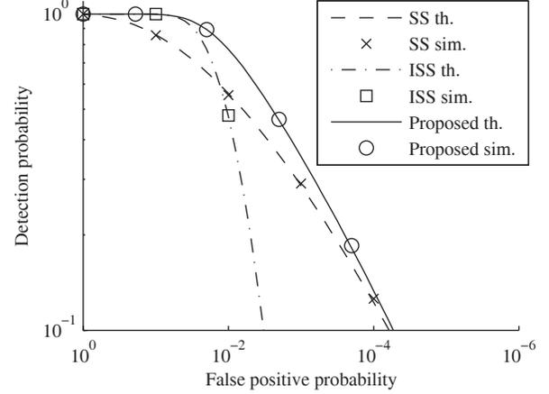
**Fig. 2.** Theoretical (th.) and simulated (sim.) ROC curves for SS, ISS ( $\lambda = 1$ ), and the proposed scheme.  $N = 8192$ ,  $\text{SWR} = 30$  dB, and  $\text{SNR} = 10$  dB.
