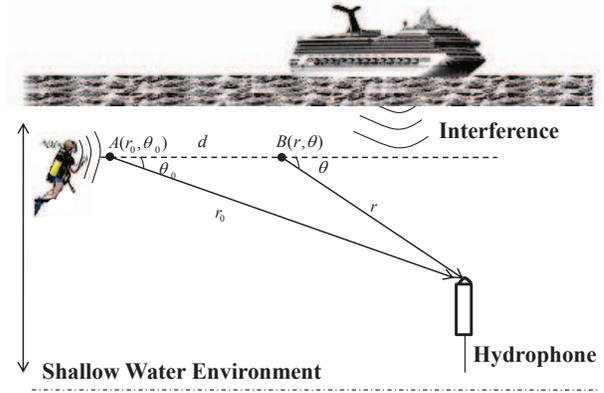
Fig. 1. Typical scenario for shallow water diver range analysis problem.
