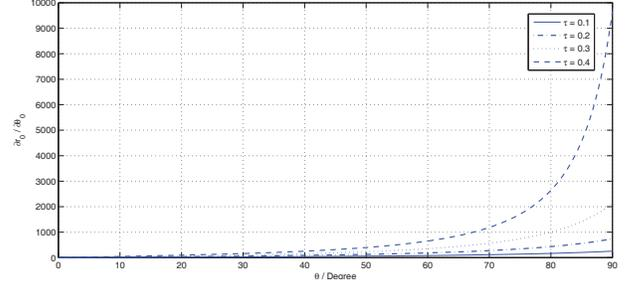
Fig. 2. The sensitivity of  $r_0$  to  $\theta_0$  for different  $\tau$ .
