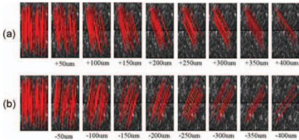
**Figure 4** The matched features between the original images (top row) and the moved images (bottom row) (a) along the +X direction (b) along the -X direction (DRT=0.6)
