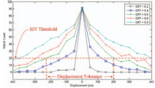
**Figure 5** The match count between the captured image and the model image using different DRT values
