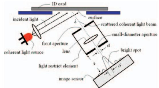
**Figure 1** The optical configuration of the proposed device
