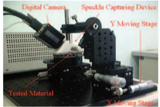
Figure 2 Experimental speckle capturing system.
