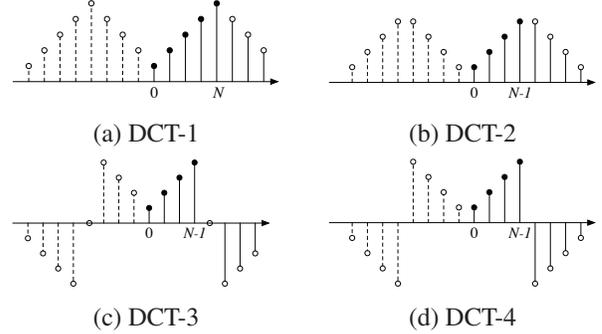
**Fig. 3.** Symmetric periodic sequence corresponding to four types of DCT. The DCT coefficients of a sequence expressed as black circles correspond to the DFT coefficients of the symmetrically extended sequence expressed as solid lines.
