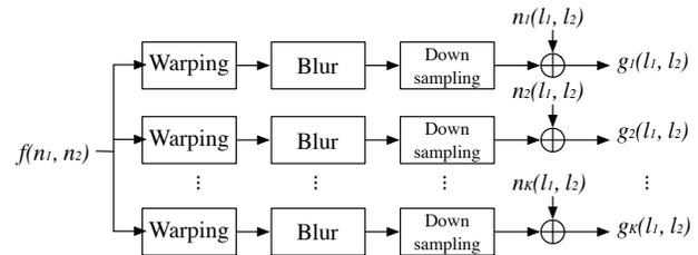
**Fig. 1.** Image acquisition model. Multiple LR images  $g_i(l_1, l_2)$  for  $i = 1, \dots, K$  are captured through a degradation process from an HR image  $f(n_1, n_2)$ .
