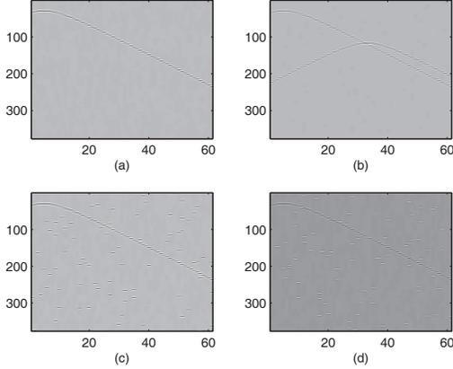
**Fig. 1.** (a) Top left: Original shot. (b) Top right: Original shot plus coherent interference (3). (c) Bottom left: Original shot plus incoherent interference (5). (d) Bottom right: Original shot plus incoherent interference (15).
