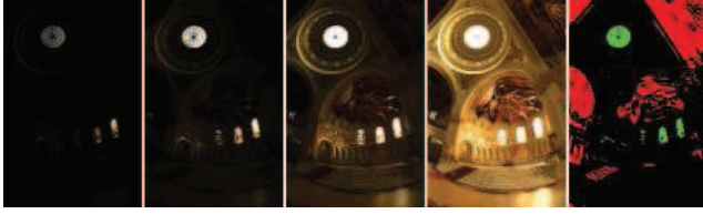
Fig. 2. Left: 4 different exposures to cover the full dynamic range of the scene in Fig. 4 (d). Selection of optimal exposure duration is outside the scope of this paper. Right (5th image): Underexposed (red) and overexposed areas (green) for the image in (c). These areas have weight zero in the SRR.
