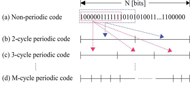
**Fig. 1.** An illustration of modulation codes for the proposed method. Each modulation codes are generated from non-periodic modulation code. (a) Non-periodic modulation code. (b) Two-cycle periodic modulation code. (c) Three-cycle periodic modulation code. (d) M-cycle periodic modulation code.
