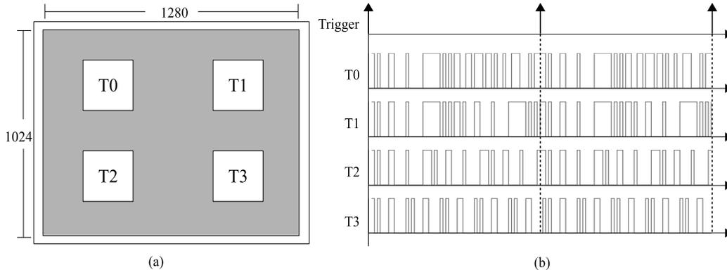
**Fig. 2.** (a)The target arrangement of this simulation. The four targets distributed as a  $2 \times 2$  matrix on the LCD monitor with a 60 Hz refresh rate and  $1024 \times 1280$  resolution. (b)The modulation codes of four targets. The trigger became positive at the interval of a stimulus cycle. The modulation code of T0 was non-periodic code, and the modulation codes of T1, T2, T2 were 2-cycle, 3-cycle and 5-cycle periodic codes.
