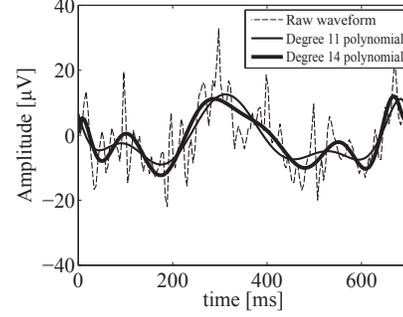
**Fig. 2.** Illustration of EEG waveform that contains P300 and its approximations to polynomial models. The fitting to the degree 11 polynomial model extracts slow waveform while fitting to the degree 14 polynomial yields more oscillations.
