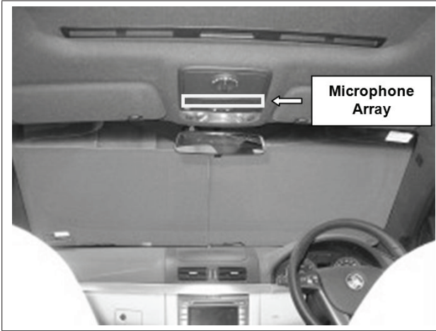
Fig. 1. Location of 8-microphone array used in Australian In-Car Speech Corpus collection.
