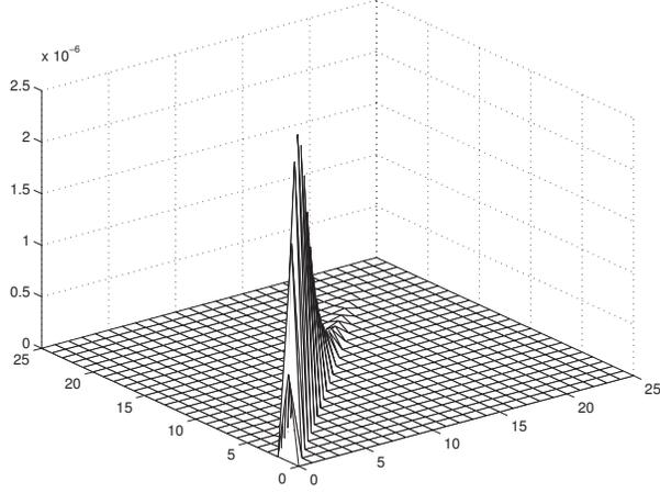
**Fig. 3:** Absolute value of matrix  $\mathbb{S}$  entries for  $\sigma = 1$ ,  $N = 2^8$  and  $M = 2N$ . Most of the energy is concentrated along the  $\sigma$ -th lower diagonal.
