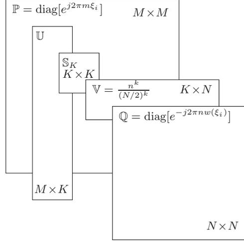
**Fig. 2:** Schematic structure of the computation of matrix  $\mathbb{A}_{M,N}$ . The resulting algorithm is fast since the total amount of multiplications is  $\propto K(M+N)$  and  $K \ll N$ .
