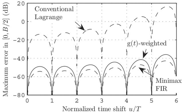
**Fig. 4.** Maximum error  $\epsilon(t)$  in band  $[0, B/2]$  versus time shift  $t$  for the conventional Lagrange and minimax FIR interpolators, and for the interpolator in (9),  $[g(t)$ -weighted interpolator].
