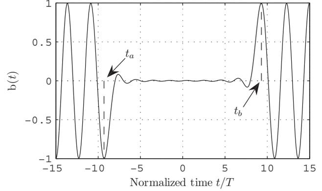
Fig. 1. Signal maximizing the interpolation error,  $b(t)$ .
