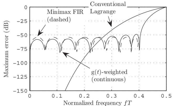
**Fig. 5.** Maximum error for time shift in  $-T/2 \leq t < T/2$  versus frequency.
