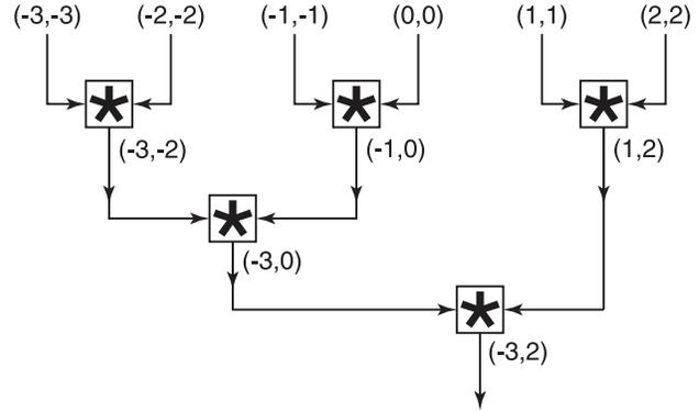
Fig. 3. Tree structure for the computation of  $(-P, P - 1)$  with  $P = 3$ . The asterisk blocks implement the operation in (17).
