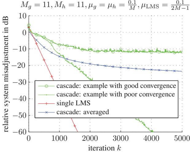
Fig. 5. Parameter error energy for cascaded LMS filters.
