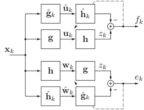
Fig. 4. Cascaded adaptive filters.
