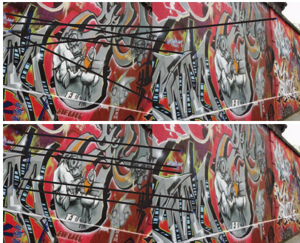
Fig. 2. Five example matches by SIFT (top) and by the proposed algorithm (bottom). The distance constraint apparently helps to fix some potential matching errors.
